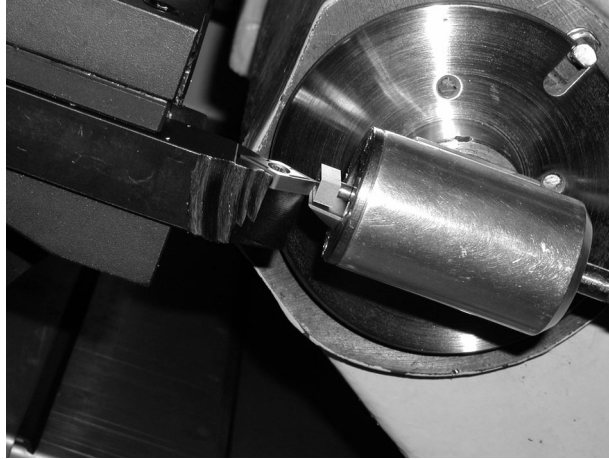
Fig. 8. The probe mounted on the tailstock of the lathe
