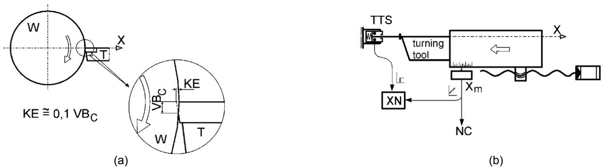
Figure 1: Geometric parameters of tool wear a) and use of a touch-trigger sensor in NC turning b)
