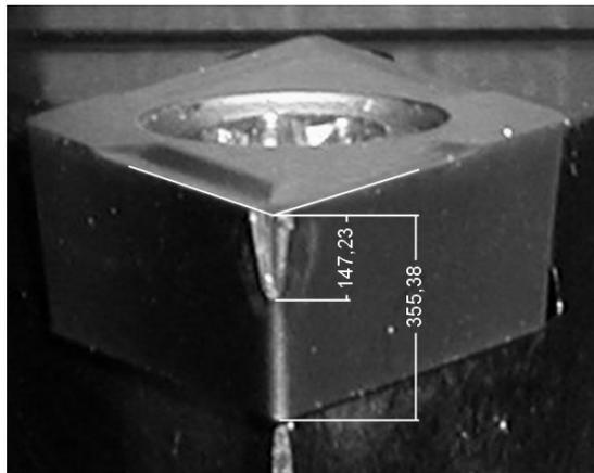
Figure 7: A picture of the insert after 5.97 min of cutting with  $v_c=250$  m/min.  $VB_c=1.64$  mm ( $KE=0.196$  mm)
