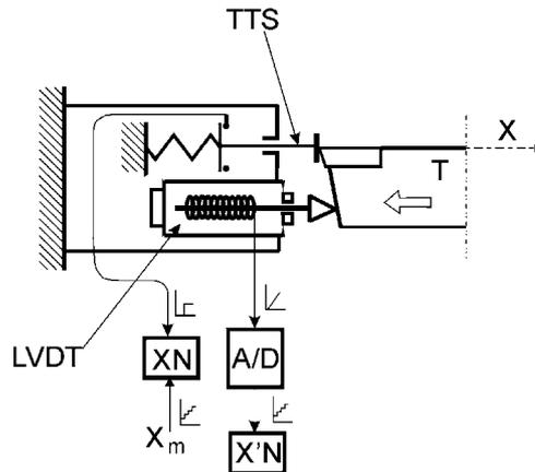
Figure 2: A tool probe with a touch-trigger sensor, TTS, and a linear variable displacement transducer, LVDT, used for the proposed method of tool wear measurement
