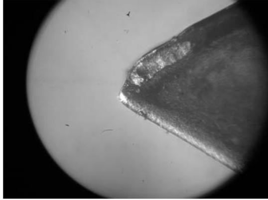
Figure 6: A cutting insert under the microscope after 33.07 min of cutting with  $v_c=100$  m/min and 150 m/min.  $KE=0.054$  mm ( $VB_c=.46$  mm)
