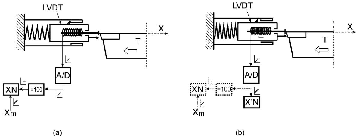
Figure 3: A probe with one LVDT: a) registration of XN, b) registration of X'N
