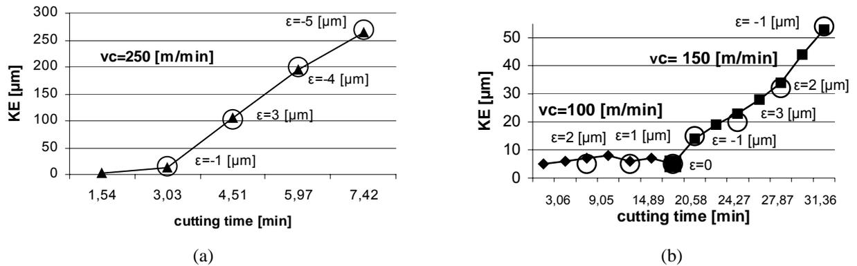
Figure 8. KE values during a test with cutting speed  $v_c = 250$  [m/min] (a); when the cutting speed was changed from  $v_c = 100$  [m/min] to  $v_c = 150$  [m/min] (b)
