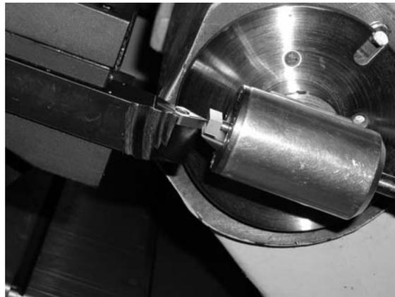
Figure 5: The probe mounted on the tailstock of the lathe
